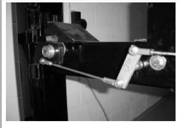
Align the flange on the 1/2" x 126" rod to approximately an 11:00 orientation. Have an assistant tighten the jam nuts tight to the coupler.
