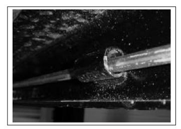
Install the 1/2" x 126" straight safety latch linkage rod into the mainside track from the opposite end. The rod should pass through two guides on the underside of the mainside track.
