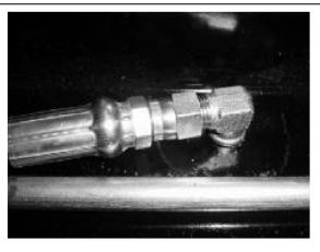
Attach one end of the other hose to the opposite side of the 90 fitting on the inside of the mainside track.
