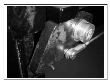
Thread a 1/4" nut to the end of the threads on each of the two eyebolts. Follow with a 1/4" washer. Install eyebolts in center of cross rail, with eye on outside of lift and secure with a 1/4" washer and nut.
