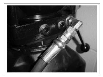
Attach the **71**" **hose** to the fitting on the power unit.
